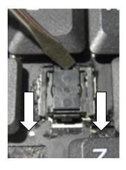
Step Four - Press key cap into place.
