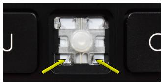
Install onto lower mounts first!
