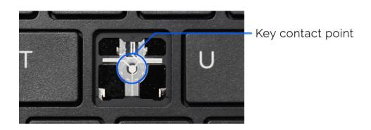
This will generally require no adhesive, as the key cap will hold the rubber cup in place when installed. If you wish to bond the new rubber cup to your keyboard, you can do so with a small amount of cyanoacrylate (also known as super glue or crazy glue - not included). Spread a *very thin* layer on the bottom surface of the rubber cup and set it into place. Allow it to dry **completely** before proceeding or you may risk damaging or inadvertently bonding other components!
